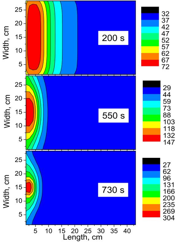
FIG. 9: Simulated temperature distributions at different time instances. Note the differences in temperature scales shown to the right.
