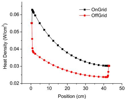
FIG. 13: Initial heat generation within the cell.
