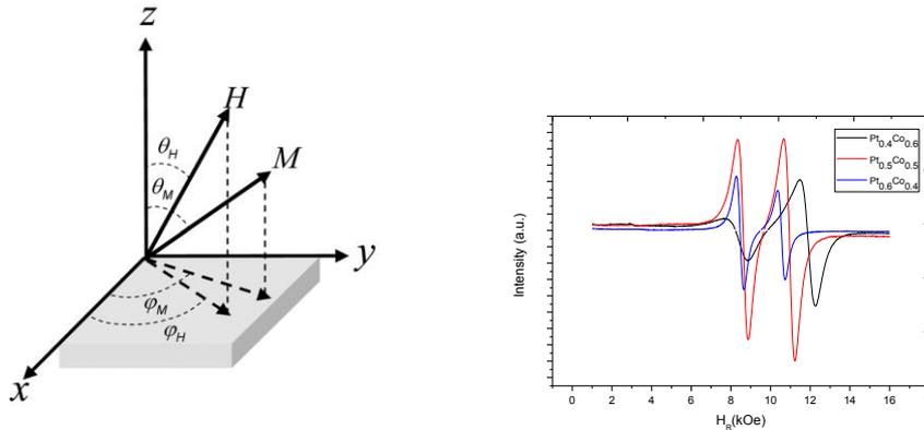
Figure-3: (a) Relative orientations of the external dc magnetic field and magnetization vectors with respect to the sample plane, (b) FMR spectra of Pt<sub>x</sub>Co<sub>1-x</sub> alloy films for the external field perpendicular to the sample plane.
