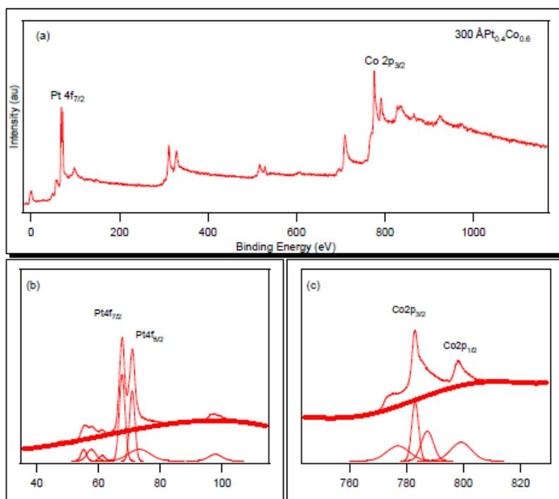
Figure-1: (a) XPS survey spectrum taken from Pt<sub>0.4</sub>Co<sub>0.6</sub> (b) The high resolution spectra for the major peak of Pt and (c) The high resolution spectra for the major peak of Co.
