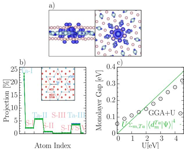
FIG. 3: a) Side- and top-views of the spin-density for monolayer  $TaS_2$ . Spin up (down) isosurfaces are indicated in blue (orange); b) atom-projected integrated charge density in the range  $[E_F - 0.1; E_F]$  for different values of the on-site electron-electron interaction  $U$  ( $U \in [0eV; 4eV]$ ), for the monolayer of  $TaS_2$ . c) Corresponding effective electron-electron interaction  $U_{\text{eff}}$  compared with the gap of the monolayer computed in DFT.
