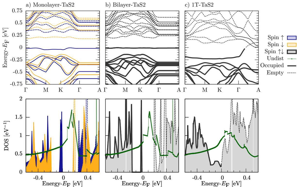
FIG. 1: Spin-resolved bandstructures (top) and density of states (bottom) for the distorted Monolayer (a), Bilayer (b), and Bulk (c) of  $TaS_2$  computed with GGA+U ( $U=2.27eV$ ) for vertically-stacked centers of distortion. The density of states for the undistorted structures are indicated with a dotted green line.
