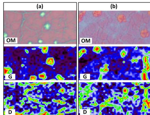
FIG. 3. Optical microscope images and Raman spectroscopy mapping on two samples with multilayer islands covered with Si (a) and multilayer graphene islands remaining uncovered after Si deposition (b). Analyzed area is  $10 \times 20 \mu\text{m}^2$ . Objective with numerical aperture of 0.85 and 514 nm laser light was used.
