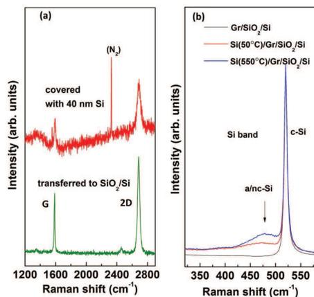
FIG. 6. (a) Raman spectra from graphene before and after Si deposition. The peak at  $2331 \text{ cm}^{-1}$  is due to atmospheric  $\text{N}_2$  which becomes visible due to long integration times. (b) Comparison of Raman Si-mode for various samples.
