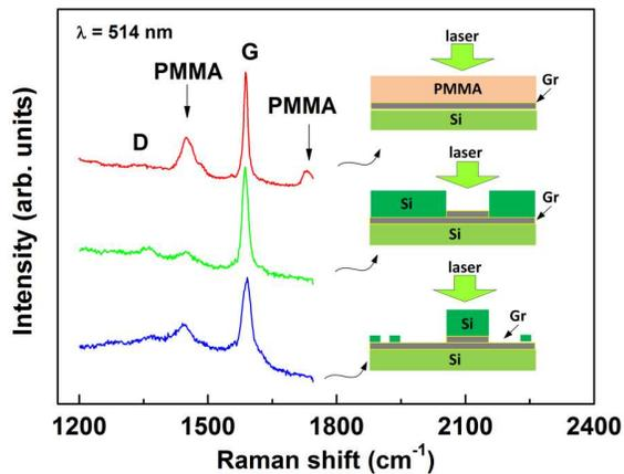
FIG. 4. Raman spectra around the G mode acquired for a reference sample before PMMA removal in acetone compared with Raman spectra from two graphene samples covered with Si. For samples covered with Si measurements were performed on Si pillars with long integration times to reveal the presence of additional features possibly related to PMMA residues.
