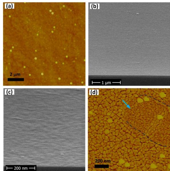
FIG. 5. (a) AFM image from a 15nm thick Si layer deposited on graphene at  $50^\circ\text{C}$ . (b-c) SEM image of a 25 nm thick Si layer deposited at  $550^\circ\text{C}$  on the low-temperature seed layer. (d) AFM phase image of the layer shown in panels b-c revealing regions with different surface topography.
