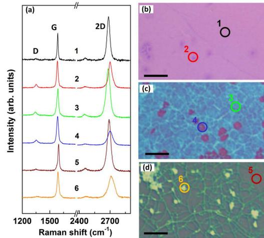
FIG. 2. (a) Raman spectra acquired from the points indicated in optical microscope images shown in panels b-d. Spectra are normalized to the same G mode intensity and vertically offset for clarity. (b) graphene after transfer. (c) after Si deposition with no Si growth on the multilayer islands. (d) after Si deposition resulting in uniform coverage of multilayer islands with Si. Scale bar in b-d is 5  $\mu\text{m}$ .
