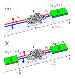
FIG. 1: (Color online) N-S and S-N-S junctions realized with helical edge states, in the presence of a ferromagnetic domain F in the normal region. The regions  $N_1$  and  $N_2$  represent the interface regions where helical states propagate freely.
