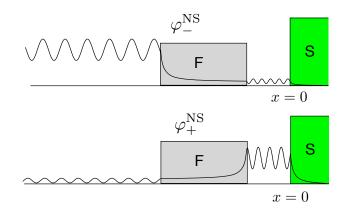
FIG. 5: (Color online) Sketch of two Majorana states, at  $\varepsilon = 0$ , in the presence of a ferromagnetic barrier. Even though they do extend on the whole normal region, they are predominently localized on one side or the other of the ferromagnetic domain (see text).
