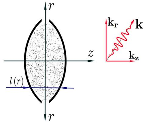
FIG. 1. (Color online) A cavity with thermostatic gaseous medium bordered by two spherically curved mirrors with a distance  $l(r)$  between them. Due to the symmetry of the system, the state space of photon inside the cavity is characterized only by longitudinal  $k_z$  and transverse  $k_r$  wave numbers.
