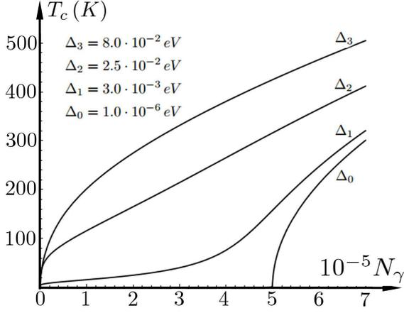
FIG. 4. Critical temperature  $T_c$  as a function of the total number of photons  $N_\gamma$  in the system, plotted according to Eq.(24) for different values of detuning parameter  $\Delta$ . The phenomenon of BEC of light demonstrates different regimes of condensation. The resonant regime ( $\Delta_0 \approx 0$ ) is desirable from the viewpoint of photon gas thermalization.
