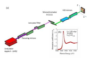
Figure 1. *a*) Experimental setup for  $\mu$ XANES measurements, performed on the dedicated-beamline LUCIA at SOLEIL. The monochromatic X-ray beam is focused on a selected spot of 2.5x2.5  $\mu$ m<sup>2</sup>, *b*) A typical La L<sub>3</sub>-edge XANES spectrum recorded in fluorescence mode on a single micrometer size spot.
