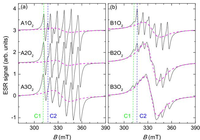
FIG. 5: Doping-dependent normalized ESR spectra of the SrTiO<sub>3</sub> samples (solid lines) at room temperature. The spectra corresponding to different concentrations are displaced for clarity. The thick dashed lines show the broad-line (C3 component) contribution to each spectrum, while the thin vertical lines indicate the lowest-field peaks of both sextets.
