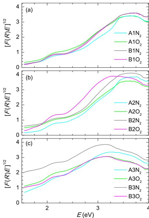
FIG. 6: The room-temperature diffuse reflectance spectra of (a) 1%, (b) 2% and (c) 3% Mn-doped SrTiO<sub>3</sub> samples.
