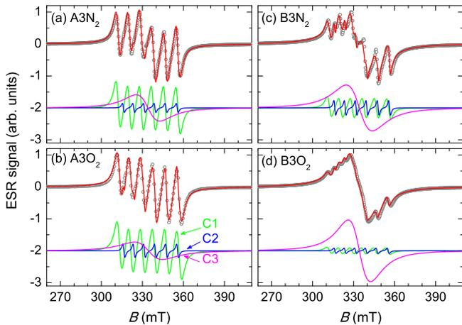
FIG. 3: The room-temperature ESR spectra of 3-% Mn-doped SrTiO<sub>3</sub> samples (circles) and their fits with a three-component model (see text for details). The three individual components are displaced vertically for clarity.
