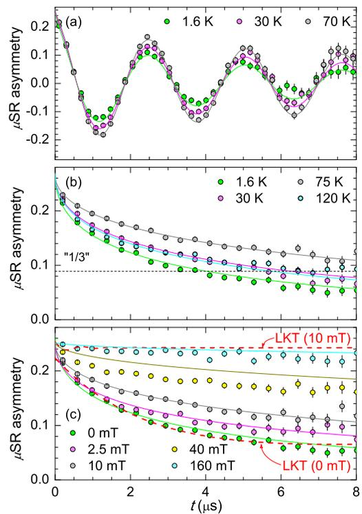
FIG. 1: The temperature-dependent  $\mu$ SR asymmetry of the A3O<sub>2</sub> sample in (a) wTF and (b) ZF. (c) Field decoupling of the longitudinal  $\mu$ SR relaxation in various LFs at 1.6 K for the same sample. The solid lines in panels (a), (b) and (c) correspond to fits to the models (4), (1) and (3), respectively. The dashed line in (b) shows the expected position of the "1/3-tail", and in (c) the prediction of the static Lorentzian Kubo-Toyabe model.
