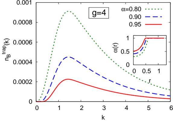
FIG. 5. (Color online) Trap-averaged bosonic momentum distribution function  $n_B^{\text{trap}}(k)$  for  $g = 4$ ,  $m_B = m_F$ , and different values of the population imbalance. Inset: local density imbalance  $\alpha(r)$ . The wave-vector  $k$  is in units of  $k_F$ , while  $r$  is in units of  $R_F$ .
