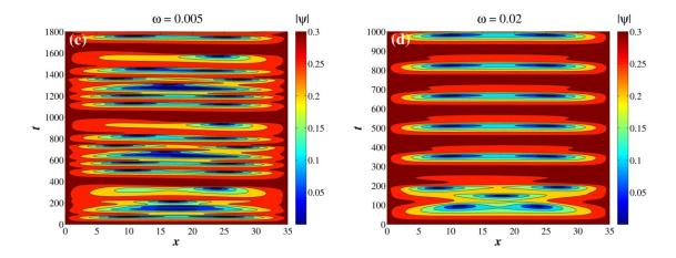
Fig. 3. Evolution (spatiotemporal dependence) of the order parameter modulus in the channel of length L = 35 for different frequencies of the applied voltage (the frequency values are shown above the panels). Voltage amplitude  $V_0 = 0.2$ . The darkest areas correspond to PSCs.
