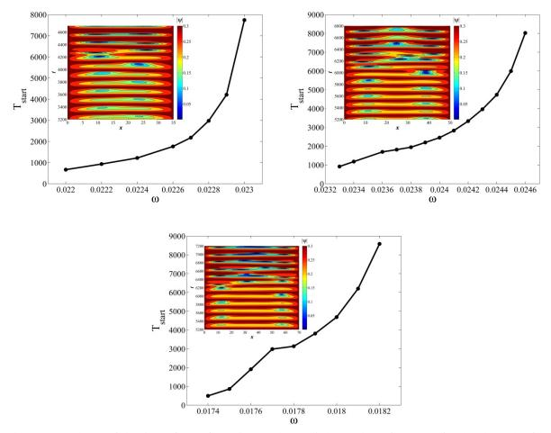
Fig. 6. Dependence of the time of PSC formation on the applied ac voltage frequency for the channels of length  $L > L^*$ : L = 35 and  $V_0 = 0.2$  (top left), L = 50 and  $V_0 = 0.3$  (top right), L = 70 and  $V_0 = 0.3$  (bottom). The insets show the evolution of the order parameter modulus for the channels of the corresponding length and at the frequency of the applied voltage  $\omega = 0.0229$  (top left),  $\omega = 0.0245$  (top right), and  $\omega = 0.0181$  (bottom).
