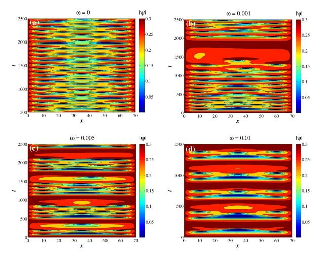
Fig. 4. Evolution (spatiotemporal dependence) of the order parameter modulus in the channel of length L = 70 for different frequencies of the applied voltage (the frequency values are shown above the panels). Voltage amplitude  $V_0 = 0.3$ . The darkest areas correspond to PSCs.
