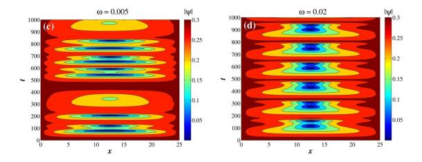
Fig. 2. Evolution (spatiotemporal dependence) of the order parameter modulus in the channel of length L = 25 for different frequencies of the applied voltage (the frequency values are shown above the panels). Voltage amplitude  $V_0 = 0.12$ . The darkest areas correspond to PSCs.
