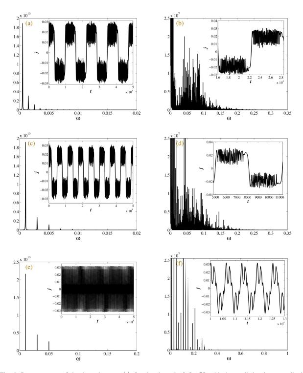
Fig. 5. Power spectra of the dependences j(t) for the channel of L = 70 with the applied voltage amplitude  $V_0 = 0.3$  and the frequencies:  $\omega = 0.0005$  (**a**),  $\omega = 0.001$  (**c**), and  $\omega = 0.01$  (**e**). Graphs (**b**), (**d**), and (**f**) show the evolution of the spectrum j(t) at higher frequencies. The insets show graphs of j(t) in a wide (**a**), (**c**), (**e**) and narrow (**b**), (**d**), (**f**) time intervals.
