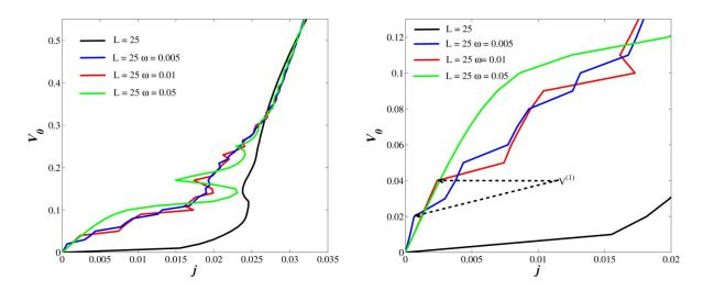
Fig. 7. CVC of the channel with L = 25 in the dc voltage (black curve) and ac voltage driven regimes for the frequencies indicated in the panel legend. On the right enlarged region of the CVC at low voltages illustrating the step-like structure of the dependences is shown. The dotted arrows show that the height of the first step in voltage  $V^{(1)}$  is equal to the quadrupled Josephson frequency (in dimensionless units) regardless of the characteristics of the applied signal (b).
