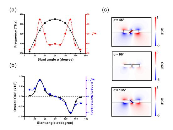
Figure 3. (a) Resonant frequency (squares, black solid line) and the field enhancement (dots, red dashed line) as functions of the slant angle of the gap. (b) Overall optical chirality enhancement (OCE, squares, black solid line) and the product of  $f_e \times \cos \alpha$  (dots, blue dashed line) as functions of the slant angle of the gap. (c) The cross sectional OCE distributions of various slant angle.
