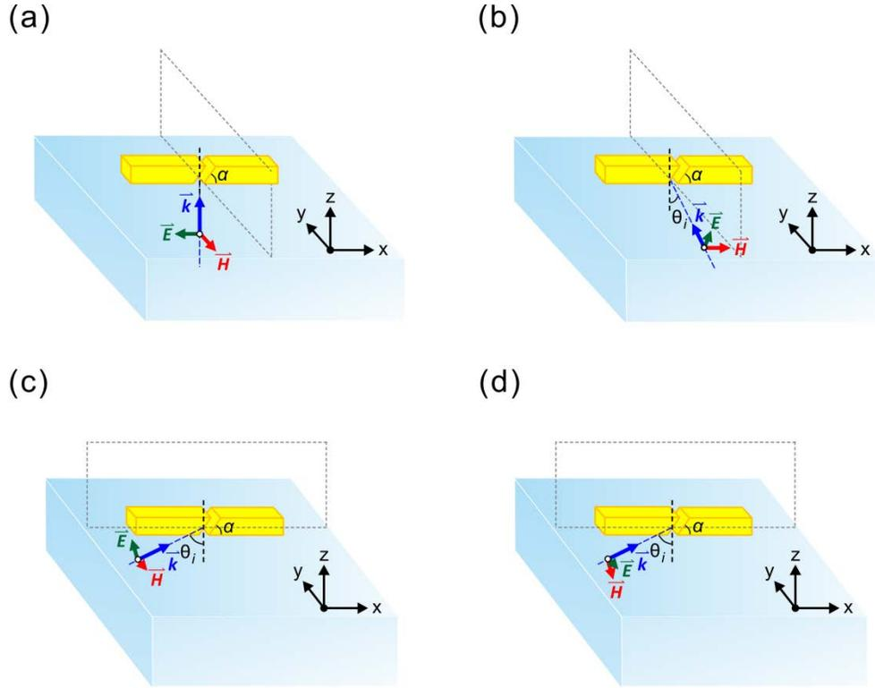
**Figure 4.** Schematic diagram of different excitation configurations, including (a) normally incident excitation linearly polarized in longitudinal antenna axis, (b) p-polarized TIR excitation with magnetic field parallel to the longitudinal axis of antenna, (c) p-polarized TIR excitation with magnetic field perpendicular to the longitudinal axis of antenna and (d) s-polarized TIR excitation with electric field component perpendicular to the longitudinal axis of antenna.
