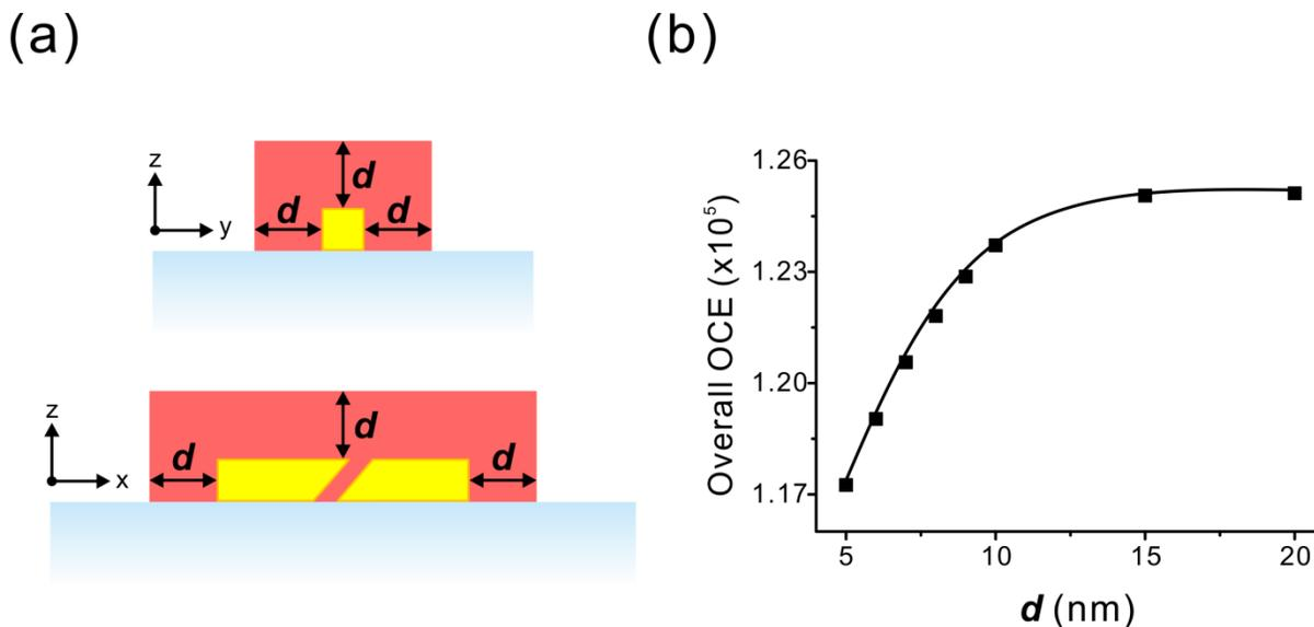
**Figure S2.** (a) The integration area (in red color) for the calculation of overall OCE. The glass half space and the area inside the antenna arms are excluded since they are not accessible to chiral matters. (b) Overall OCE value as a function of  $d$  for the 160-nm antenna at the fundamental resonance. Solid line is a guide line for the eye.
