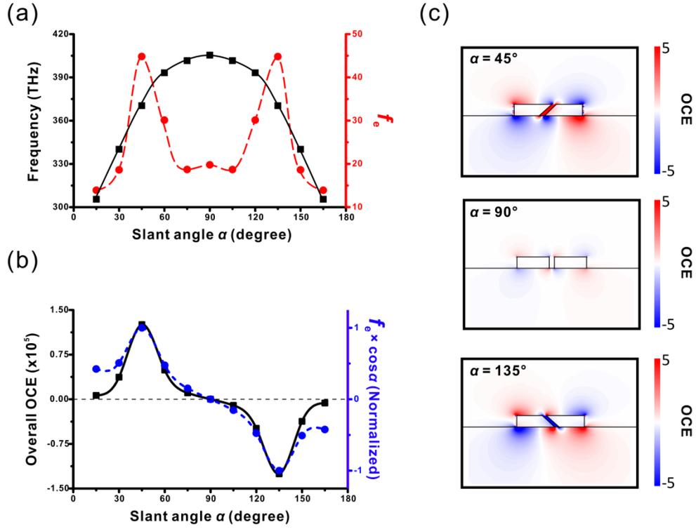
**Figure 3.** (a) Resonant frequency (squares, black solid line) and the field enhancement (dots, red dashed line) as functions of the slant angle of the gap. (b) Overall optical chirality enhancement (OCE, squares, black solid line) and the product of  $f_e \times \cos\alpha$  (dots, blue dashed line) as functions of the slant angle of the gap. (c) The cross sectional OCE distributions of various slant angle.
