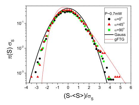
FIG. 6: (Color online) Normalized probability density function of the intensity fluctuations detected in a hybrid cell for the power  $P\sim0.7$ mW of the incoming light at different polarization directions (as denoted in the legend) in the reverse geometry. The solid lines represent the Gaussian and the gFTG distribution without any fit parameter.
