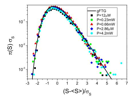
FIG. 5: (Color online) Normalized probability density function of the intensity fluctuations detected in a planar cell for the polarization  $\alpha = 45^{\circ}$  at different powers of the incoming light (as denoted in the legend) in the reverse geometry. The solid line represents the gFTG distribution without any fit parameter.
