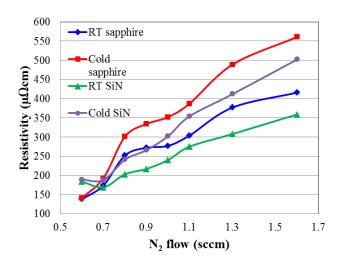
Fig.5. Room temperature (RT) and 20 K (cold) resistivity as a function of nitrogen flow rate.
