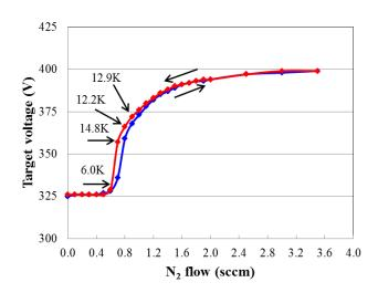
Fig. 1. The target voltage as a function of nitrogen flow with a constant argon flow of 16.2 sccm and power of 100 W. The  $T_c$ 's of NbN films deposited at the four operating points on the hysteresis curve are shown.
