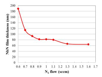
Fig.4. NbN film thickness as a function of nitrogen flow rate.
