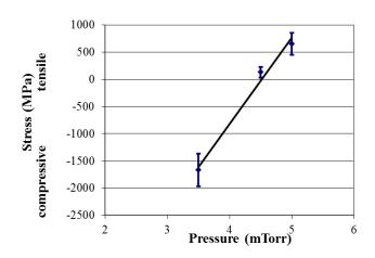
Fig.8. Film stress for argon deposition pressures of 3.4 mT, 4.5 mT and 5mT.
