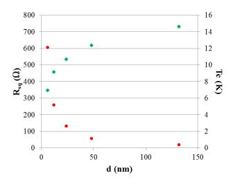
Fig. 12. Square resistance and transition temperature as a function of film thickness: 6 nm, 12 nm, 24 nm and 48 nm films were used.
