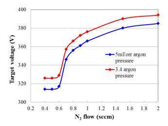
Fig.3. Niobium target voltage as a function of flow rate, on the decreasing branch of the hysteresis curve for argon pressures of 3.4 mT and 5.0 mT
