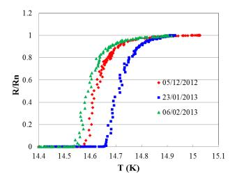
Fig. 11. Normal resistance verses temperature for films deposited with notionally identical conditions. The measured  $T_c$ 's were 14.59K (green), 14.63K (red) and 14.67K (blue). The RT resistivity and RRR were 217  $\mu\Omega$ cm and 0.84 (green), 229  $\mu\Omega$ cm and 0.82 (red), 237  $\mu\Omega$ cm and 0.81 (blue).
