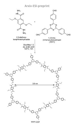
**Scheme S5.** Synthesis of TFPT-COF by acid catalyzed hydrazone formation.
