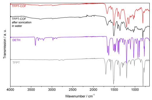
Figure S17. FT-IR spectra showing the almost unchanged vibrational pattern of TFPT-COF before and after water exposure.
