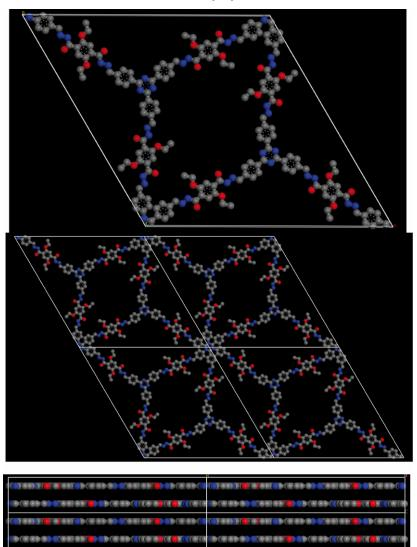
**Figure S8.** Simulation of the crystal structure with staggered arrangement of adjacent layers: Top view onto the *ab*-plane and view perpendicular to the *c*-axis showing the doubled stacking period due to the staggered AB layer arrangement.
