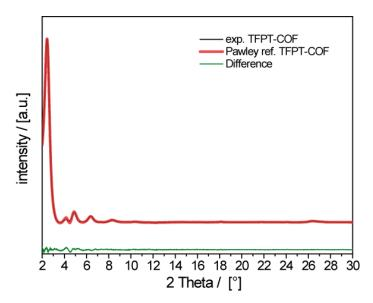
Figure S7. Experimental powder pattern and Pawley refined pattern based on P1 symmetry.
