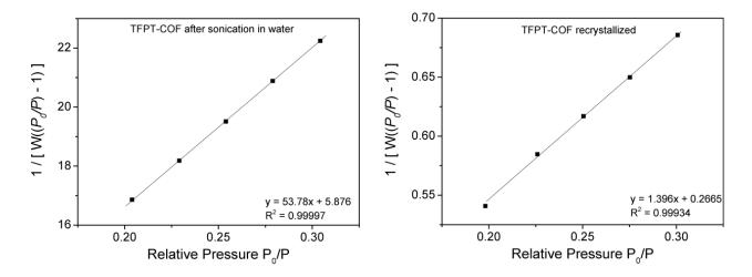
Figure S18. Linear BET plot of TFPT-COF after H<sub>2</sub>O exposure and TFPT-COF (recrystallized) as obtained from Ar adsorption data at 87 K.
