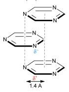
Figure S9. Shift (parallel displacement) in a zig-zag manner to minimize electrostatic repulsion between adjacent layers.
