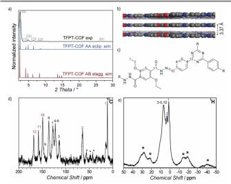
**Fig. 2** Characterization of the TFPT-COF by PXRD and MAS solid-state NMR spectroscopy. (a) and (b) PXRD suggests a (close to) eclipsed layer stacking as confirmed by Pawley refinement of the AA-stacked structure model. c) Assignment of  $^{13}$ C and  $^{1}$ H NMR data. (d)  $^{13}$ C CP-MAS NMR spectrum, asterisks mark spinning side bands. (e)  $^{1}$ H MAS NMR spectrum with a group of signals centered between 1 and 8 ppm; asterisks mark spinning side bands.
