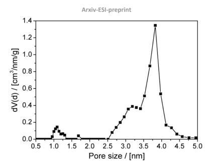
Figure S13. Pore size distribution calculated based on NLDFT using the "Ar-zeolite/silica cylindrical pores at 87 K" kernel.
