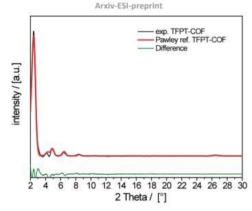
Figure S6. Experimental powder pattern and Pawley refined pattern based on P6/m symmetry.
