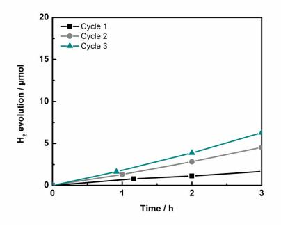
**Figure S20.** Cycle measurements of TFPT-COF for 95 h with ascorbate as sacrificial donor ("Cycle" corresponds to centrifugation and resuspending in ascorbate containing water).
