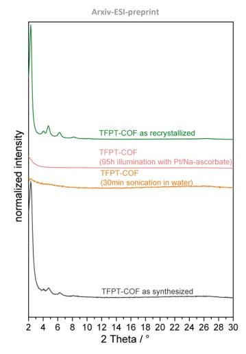
**Figure S16.** PXRD patterns of TFPT-COF, showing loss of crystallinity after water exposure and photocatalysis. The TFPT-COF can be obtained by recrystallization.
