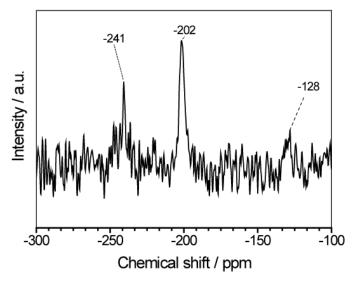
Figure S4. <sup>15</sup>N CP-MAS spectrum of TFTP-COF.
