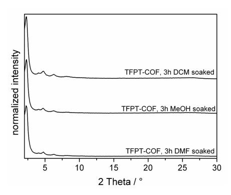
Figure S15. PXRD measurements showing the retention of crystallinity after treatment with different solvents.
