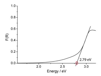
Figure S14. Plot of Kubelka-Munk function used for band gap extraction.
