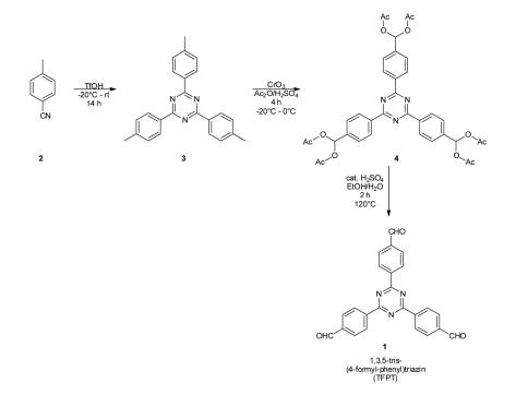
Scheme S1. Synthesis of 1,3,5-tris-(4-formyl-phenyl)triazine (TFPT) (1) by a three-step modified literature procedure.<sup>52</sup>
