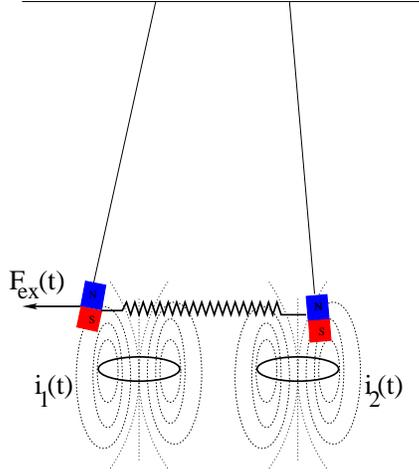
Figure 1: Sketch of the physical system under consideration. Each pendulum contains a magnet and the modulation of its natural oscillation frequency is controlled by the time-dependent current  $i_{1,2}(t)$  flowing in the corresponding coil. The first pendulum may be externally driven by a time-dependent force  $F_{\text{ex}}(t)$ .
