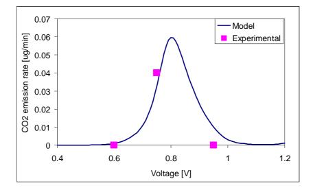
Figure 3: Steady state emission of CO<sub>2</sub> as a function of potential
