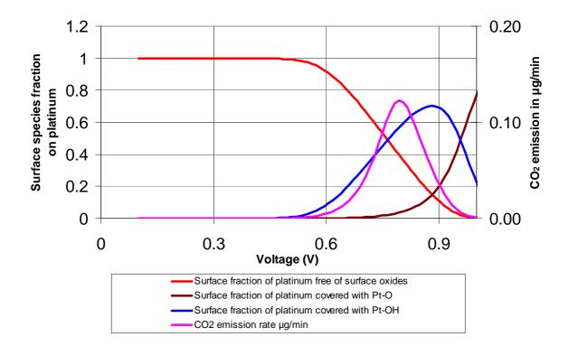
Figure 5: Steady state coverage of species on platinum surface as a function of potential
