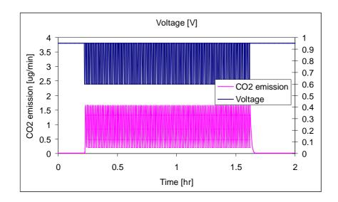
Figure 9: Model prediction of Carbon corrosion under 30s/20s voltage cycle between 0.6 V and
