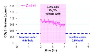
Figure 10. Experimental data of  $CO_2$  emission response to 30 s / 20 s voltage cycle between 0.6 V and 0.95 V (75°C, 95% RH, 0.15 slpm H<sub>2</sub> & 0.36 slpm N<sub>2</sub>)
