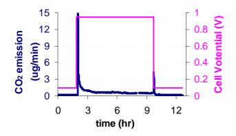
Figure 7: Experimental data of CO<sub>2</sub> emission response to step changes in voltage Testing conditions: cell = 75°C. Anode & cathode = 95% RH, 0.15SLPM  $H_2$  & 0.36SPLM  $N_2$
