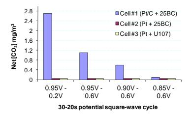
Figure 1. Increment of CO<sub>2</sub> concentration in cathode exhausts during the potential square-wave cycling (50s/cycle, 30s at upper voltages and 20s at low voltages)
