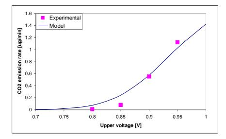
Figure 11: Comparison of the model predictions and experimental data on the impact of the upper voltage on carbon corrosion: 30 s / 20 s cycling, lower voltage = 0.6 V, at RH = 0.95
