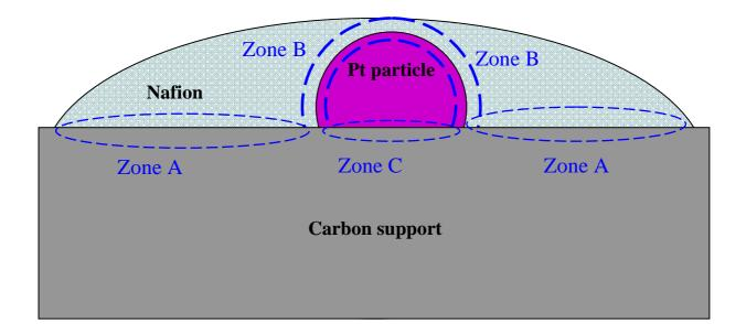
Figure 2: Schematic of the cathode catalyst layer
