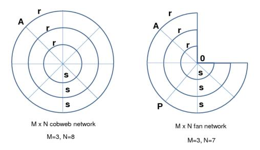
FIG. 1: An  $M \times N$  fan network with M=3 and N=7 (right). Bonds in the radial and circular directions comprise resistors s and r. The apex point is denoted by O, A denotes any point on the boundary and P denotes a point at the middle of the boundary. We also show  $M \times N$  cobweb network with M = 3 and N = 8 (left)
