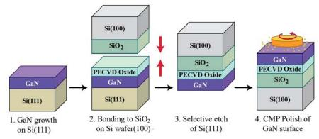
Fig. 1. GaN photonic circuits are built on GaN on silicon dioxide on silicon (GaNOI) substrates. The GaNOI substrate fabrication process runs as follows: PECVD oxide is first deposited onto commercially available GaN on Si (111) wafers to assist the bonding process; the Si (111) layer is removed after the bonding and the new GaN surface undergoes CMP.
