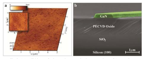
Fig. 2. a) An AFM image of a 5  $\mu$ m × 5  $\mu$ m area showing rms roughness of 4 nm on the polished GaN surface; (b) a cross sectional scanning electron micrograph showing a fabricated GaN waveguide (in false-color), oxide layers and the silicon (100) substrate. The trapezoidal profile of the waveguide is due to the anisotropy of the RIE process.
