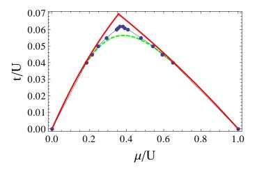
FIG. 2: (Color online) Phase boundary of a 2D square lattice for  $J_0 (A/(\hbar\omega)) = 0.4$ : third-order strong-coupling expansion result according to (36), (37) (red solid line), QMC result in the thermodynamic limit (blue line dot), and second-order EPLT result (35) (green dashed line).
