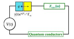
FIG. 1: Extended tunneling between arbitrary similar or different conductors with mutual (thus capacitive) or internal Coulomb interactions, disorder, superconducting correlations, and coupling to other quantum systems and an electromagnetic environment with impedance  $Z(\omega)$ . Tunneling amplitudes scan depend on many-body states  $\alpha$ , as well as on time through an arbitrary complex function  $\gamma(t)e^{iqV_T t}$ , which is the case for TD local magnetic field and gate voltage
