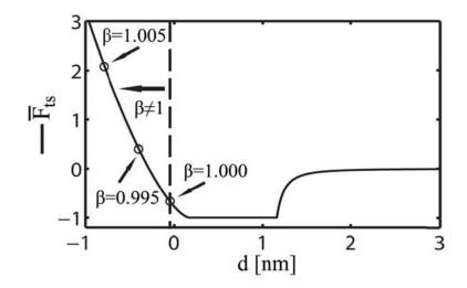
FIG. 3 Variation of fundamental drive frequency  $\beta$  under SASS. Numerical integration predicts that the minimum distance of approach can be varied for a given  $\bar{A}_1$  (here 0.2) and  $A_0$  (here 1 nm) as a function of fundamental (normalized) drive frequency  $\beta$  when the tip is in perpetual contact with the water layer (SASS).
