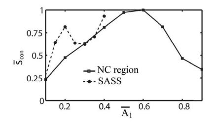
FIG. 10 Numerically calculated sensitivity (normalized)  $S_{con}$  of the second mode phase shift  $\Delta \phi_2$  to variations in conservative sample properties in the NC (continuous lines) and SASS (dashed lines) regions. The parameters as the same as those in Fig. 8. Maxima was  $S_{con}\approx99.7$  [°/N/m].
