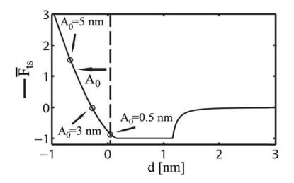
FIG. 5 Variation of fundamental free amplitude under SASS. Numerical integration predicts that the mechanical contact region can be accessed and that the minimum distance of approach d can be decreased for a given  $A_1$  (here 0.2 nm) with decreasing  $A_0$  in SASS. Here  $\beta=1$ .
