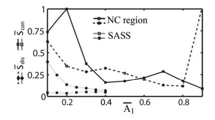
FIG. 11 Numerically calculated sensitivity (normalized)  $S_{dis}$  in the NC (dashed lines and circle markers) and SASS (thin dashed lines and circle markers) regions in the presence of dissipative variations in sample properties only. The signal  $S_{con}$  has also been plotted with continuous lines and square markers and thin dashed lines and square markers in the NC and SASS regions respectively. Maxima was  $S_{dis}\approx 1092$  [°/eV].
