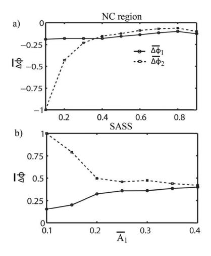
FIG. 9 Numerically calculated difference (normalized) in phase shift response of the first  $\Delta \phi_1$  (continuous lines) and second  $\Delta \phi_2$  modes (dashed lines) as a function of normalized amplitude  $\bar{A}_1$ . Dissipative variations only are allowed in the interaction in (a) the NC (maxima of  $\Delta \phi_2 \approx 14.2^\circ$ ) and (b) SASS (maxima of  $\Delta \phi_2 \approx 6.9^\circ$ ) regions.
