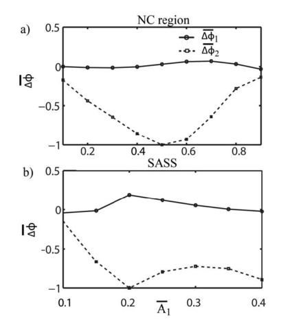
FIG. 8 Numerically calculated difference (normalized) in phase shift response of the first  $\Delta \phi_1$  (continuous lines) and second  $\Delta \phi_2$  modes (dashed lines) as a function of normalized amplitude  $\bar{A}_1$ . Conservative variations only are allowed in the interaction in (a) the NC (maxima of  $\Delta \phi_2 \approx 3.3^\circ$ ) and (b) SASS (maxima of  $\Delta \phi_2 \approx 10.2^\circ$ ) regions.
