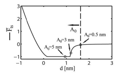
FIG. 4 Variation of fundamental free amplitude under standard small amplitude operation  $\bar{A}_1$ =0.9. Numerical integration predicts that the minimum distance of approach can be varied for a given  $\bar{A}_1$  (here 0.9) as a function of  $A_0$  when driving exactly at  $\beta$ =1.
