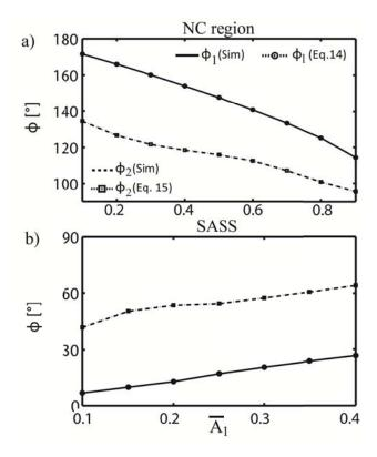
FIG. 7 Numerically calculated (Sim ) response of the fundamental shift  $\phi_1$  (continuous lines) and the second mode shift  $\phi_2$  (dashed lines) as a function of normalized amplitude  $\bar{A}_1$  in the (a) NC region and the (b) SASS region. Comparisons with analytical expressions are shown. The interaction includes dissipation.
