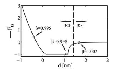
FIG. 2 Variation of fundamental drive frequency  $\beta$  under standard small amplitude operation  $\bar{A}_1$ =0.9. Numerical integration predicts that the minimum distance of approach can be varied for a given  $\bar{A}_1$  (here 0.9) and  $A_0$  (here 1 nm) as a function of fundamental (normalized) drive frequency  $\beta$ .
