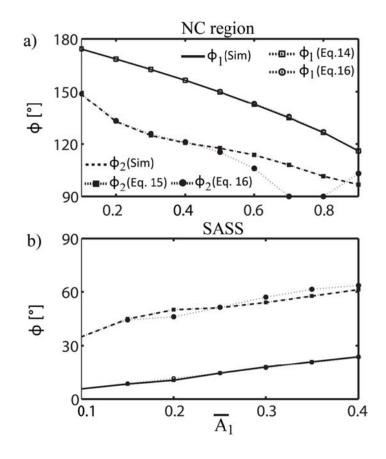
FIG. 6 Numerically calculated (Sim ) response of the fundamental shift  $\phi_1$  (continuous lines) and the second mode shift  $\phi_2$  (dashed lines) as a function of normalized amplitude  $\bar{A}_1$  in the (a) NC region and the (b) SASS region. Comparisons with analytical expressions are shown. The interaction is conservative.
