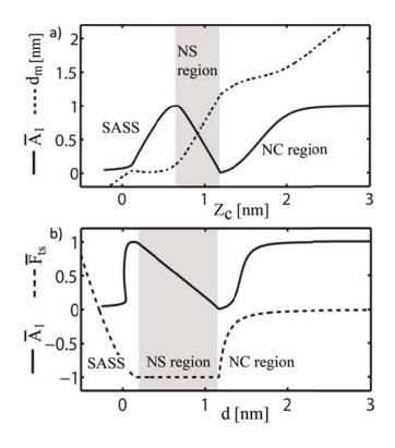
FIG. 1 (a) Response of the fundamental amplitude  $\bar{A}_1$  (continuous lines) and the minimum distance of approach  $d_m$  (dashed lines) as a function of separation  $z_c$  with the use of small amplitudes  $A_0=0.5$  nm. (b) Relationship between  $\bar{A}_1$  and  $d_m$  or d, i.e.  $\bar{A}_1(d)$ . The actual tip-sample (normalized) force  $F_{ts}$  (dashed lines) is also plotted for comparison.
