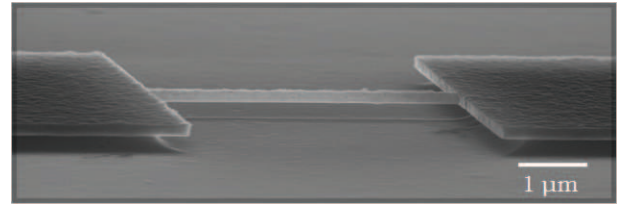
FIG. 1: Scanning electron micro-graph of a diamond resonator. The dimensions of the resonator are 480 nm x 300 nm (width x thickness). Different resonators with different lengths ranging from 5 to 30 \mu m have been fabricated.
