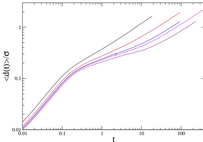
Figure 4. Mean distance traveled by an atom versus time for a Lennard-Jones system of 1000 particles on  $S^2$  at a reduced density  $\rho = 0.92$  and various temperatures  $T = 2, 1.6, 1.2, 0.9, 0.8$  (from top to bottom).
