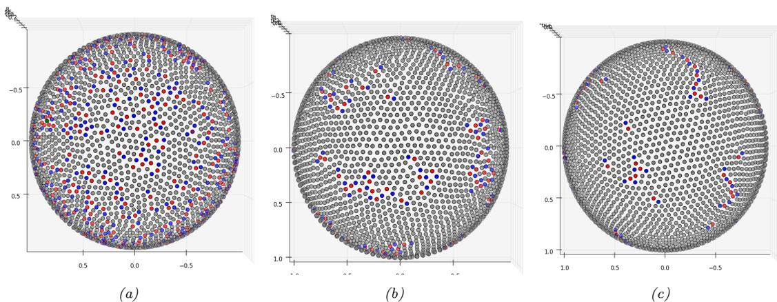
Figure 2. Typical atomic configurations at different temperatures: (a)  $T = 2$ , (b)  $T = 1$  and (c)  $T = 0.5$ . Red particles correspond to 7 neighbors (negative disclination), blue particles to 5 particles (positive disclination) and grey particles to 6 neighbors.
