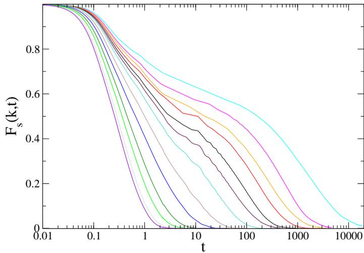
Figure 3. Log-linear plot of the self-intermediate scattering function  $F_s(k, t)$  of a Lennard-Jones system of 1000 particles on  $S^2$  at a reduced density  $\rho = 0.92$  for various temperatures  $T = 3, 2.5, 2, 1.6, 1.2, 1, 0.8, 0.7, 0.6, 0.55, 0.5, 0.4$  (from left to right).
