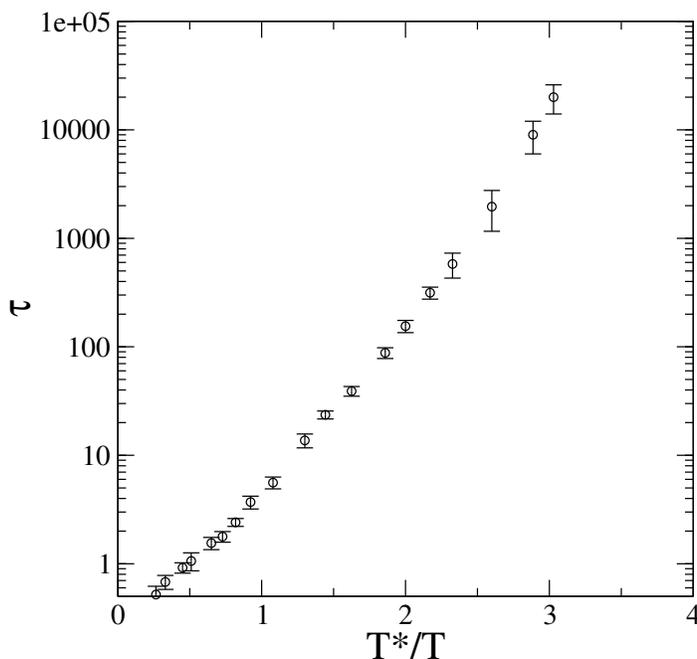
Figure 5. Arrhenius plot of the relaxation time  $\tau$  versus the reduced inverse temperature  $T^*/T$ , where  $T^* \approx 1.3$  is an estimate of the temperature at which ordering in a hexagonal phase takes place in the Euclidean plane. The parameters are the same as in Fig. 3.
