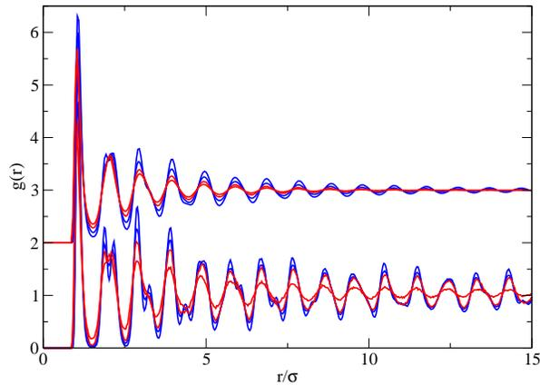
Figure 1. Pair correlation function  $g(r)$  as a function of the (geodesic) distance  $r$  for a Lennard-Jones system of 1000 particles at a reduced density  $\rho = 0.92$  and for temperatures  $T$  from 2 (red) down to 0.8 (blue). The top curves are for the sphere  $S^2$  (results shifted by a step of 2) and the bottom curves are for the Euclidean plane  $E^2$  with periodic boundary conditions.
