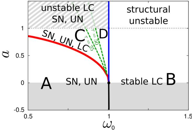
Figure 4. (Color online) Dynamical regimes in the  $(\omega_0, a)$  parameter space for  $\tau \rightarrow \infty$ . Capital letters name the excitable (A), the oscillatory (B), and the bistable regime (C and D). Topological properties are denoted by SN (stable node), UN (unstable node), and LC (limit cycle). Thick lines indicate bifurcations between different regimes, dashed lines bifurcations that occur for finite  $\tau$ , and the dotted line separates the region where trajectories diverge.
