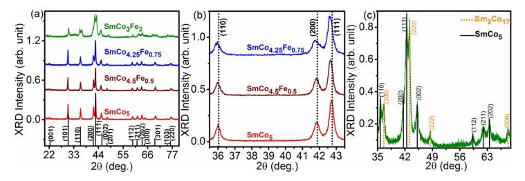
**Fig.1. a)** XRD of  $SmCo_{5-x}Fe_x$  for x=0, 0.5, 0.75 and 2 compared with prototype  $CaCu_5$ -structure (vertical lines). **b)** Expanded view of the XRD showing left shift of the peaks with respect to  $SmCo_5$  (vertical dotted lines) due to Fe addition. **c)** XRD of  $SmCo_3Fe_2$  showing mixture of  $SmCo_5$  (vertical solid lines) and  $Sm_2Co_{17}$  (vertical dotted lines) phases.
