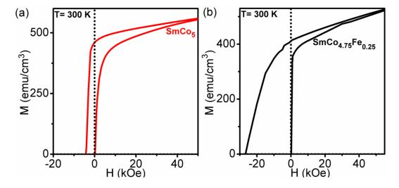
**Fig. 3.** Virgin M vs. H graph for **a**) SmCo<sub>5</sub> and **b**) SmCo<sub>4.75</sub>Fe<sub>0.25</sub>. The slope of the virgin plot region for b) is higher than a) showing domain wall nucleation effect induced by Fe addition.
