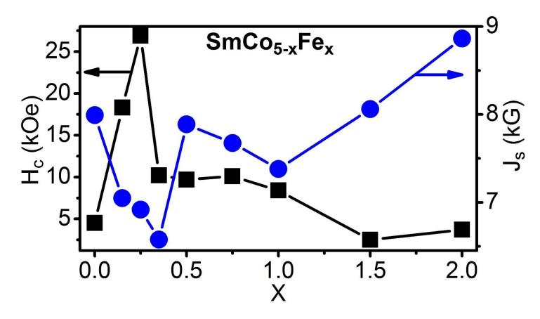
**Fig. 4.** Magnetic properties of  $SmCo_{5-x}Fe_x$  for a range of x between 0 and 2.
