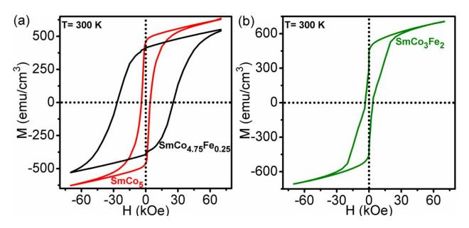
**Fig. 2. a)** Magnetization (M) vs. applied magnetic field (H) plots for SmCo<sub>5</sub> and SmCo<sub>4.75</sub>Fe<sub>0.25</sub> showing improvement of coercivity with Fe addition. **b)** M-H hysteresis loop of SmCo<sub>3</sub>Fe<sub>2</sub> exhibiting hard-soft two phase characteristic.
