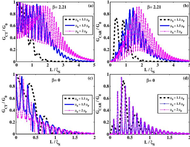
FIG. 6. (Color online) Charge conductance of the CT and CAR processes as a function of  $L/\xi_S$  for different values of the chemical potential  $\mu_S$  in MoS<sub>2</sub>-based structure with  $\alpha = 0$ ,  $\beta = 2.21$  (a)-(b) and  $\beta = 0$  (c)-(d), when  $\Delta = 1.9$  eV,  $\mu_F = -\Delta/2 + \lambda - h + eV + 0.001$ ,  $\Delta_S = 0.05$  eV,  $h = 0.5\lambda$  and  $eV/\Delta_S = 0$ .
