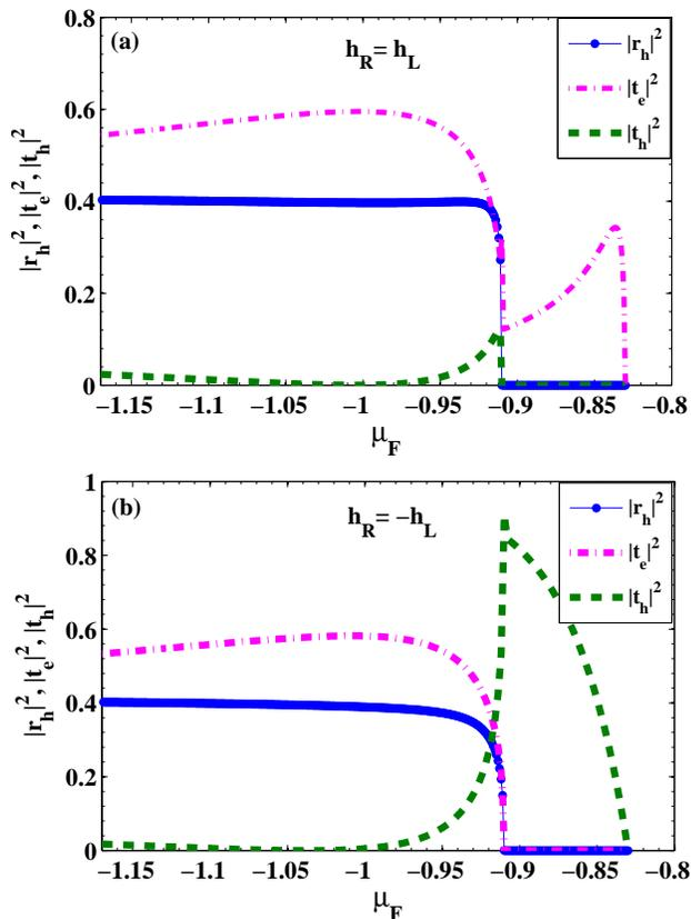
FIG. 2. (Color online) Probabilities of the AR ( $|r_h|^2$ ), CT ( $|t_e|^2$ ) and CAR ( $|t_h|^2$ ) processes as a function of the chemical potential of the F region,  $\mu_F$ , for normal incidence ( $\theta_e = 0$ ) to the MoS<sub>2</sub>-based F/S/F structure with (a) parallel ( $h_R = h_L$ ) and (b) antiparallel ( $h_R = -h_L$ ) alignments of magnetizations, when  $h_L = 0.5\lambda$ ,  $L/\xi_S = 0.5$ ,  $\mu_S = -1$  eV, and  $eV/\Delta_S = 0$ .
