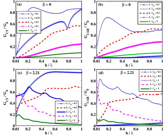
FIG. 7. (Color online) Dependence of the charge conductance of the CT and CAR processes on the magnitude of the exchange field in the right F region  $|h_R|/\lambda = h/\lambda$  (in units of the spin-orbit coupling constant  $\lambda$ ) for different lengths of the S region, when  $\beta = 0$  (a)-(b) and 2.21 (c)-(d),  $\alpha = 0$ ,  $eV/\Delta_S = 0$ ,  $\mu_F = -\Delta/2 + \lambda + eV - 0.001$ ,  $\mu_S = 1.1 \mu_F = -1$  eV and  $\Delta_S = 0.01$  eV.
