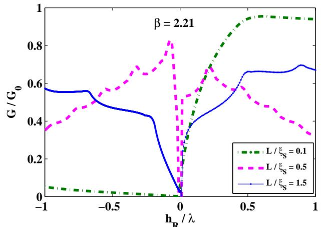
FIG. 3. (Color online) Cross-conductance of the superconducting spin valve structure versus the exchange field of the right F region  $h_R/\lambda$  (in units of the spin-orbit coupling constant  $\lambda$ ) for three different lengths of the S region, when  $\alpha = 0$ ,  $\beta = 2.21$ ,  $eV/\Delta_S = 0$ ,  $\mu_F = -\Delta/2 + \lambda + eV - 0.001$ ,  $\mu_S = 1.1$   $\mu_F = -1$  eV and  $\Delta_S = 0.01$  eV.
