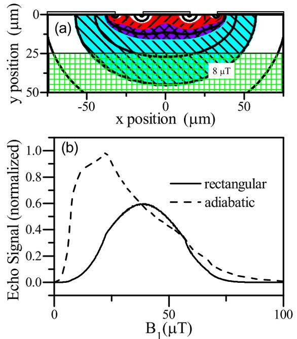
FIG. 4. (a) Cross section of resonator at an antinode in  $B_1$  with contour lines indicating  $B_1$  magnitude for a 400 nW input power. The hatched regions denote the location of spins contributing to 2/3 of the echo intensity for rectangular (red) pulses and adiabatic (blue) pulses (violet where they overlap). The green-hatched region below  $25 \mu\text{m}$  denotes the undoped portion of the sample. (b) Plot of the echo intensity contribution of all spins at particular values of  $B_1$ .
