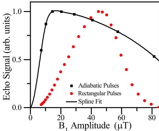
FIG. 3. Plot of echo amplitude as a function of  $B_1$  for a sample in a high-homogeneity resonator with adiabatic pulses (black) and rectangular pulses (red). Data were taken at 4.6 K in a DC magnetic field of 0.34 T. The solid line is a spline fit to the data and is used later in a simulation.
