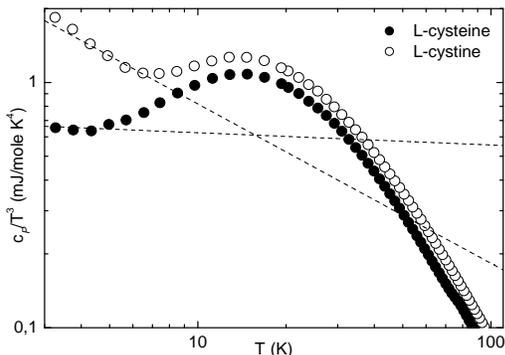
FIG. 4.  $c_p/T^3$  vs  $T$  specific heat data of L-cysteine (closed circles) and L-cystine (open circles). Dashed lines represent the TLS contribution  $\propto T^{-0.005}$  and  $\propto T^{-0.65}$  for L-cysteine and L-cystine, respectively.
