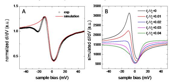
Fig. S1 (A) The experimental dI/dV curve measured at 5 K and the simulated curve using the co-tunneling model with  $t_f/t_c = 0.013$ . (B) Co-tunneling simulations using different values of  $t_f/t_c$ .
