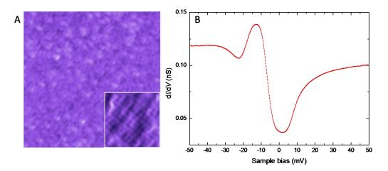
Fig. S4 (A) A 600 Å × 600 Å topography on the "A2" phase. The inset shows a 50 Å × 50 Å area with atomic resolution, where the atoms form a 4 Å × 4 Å square lattice. (B) The spatially averaged dI/dV spectrum in this area.
