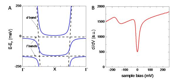
Fig. S3 (A) Illustration of the hybridization process. The itinerant *d*-band interacts with the two flat *f*-bands. (B) The simulated large energy range spectrum reproduces the hump feature at  $\sim -160$  meV.
