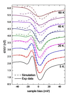
Fig. S2 Thermal broadening simulation at different temperatures. We take the T = 5 K curve and do thermal convolution for higher temperatures. The thermal effect is too weak to suppress the resonance peak feature up to 60 K.
