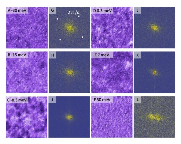
Fig. S6 (A)~(F) The dI/dV map at several representative bias voltages on another 200 Å × 200 Å area. (G)~(L) The corresponding FT of each dI/dV map. The small white dots indicate the Bragg points of the lattice.
