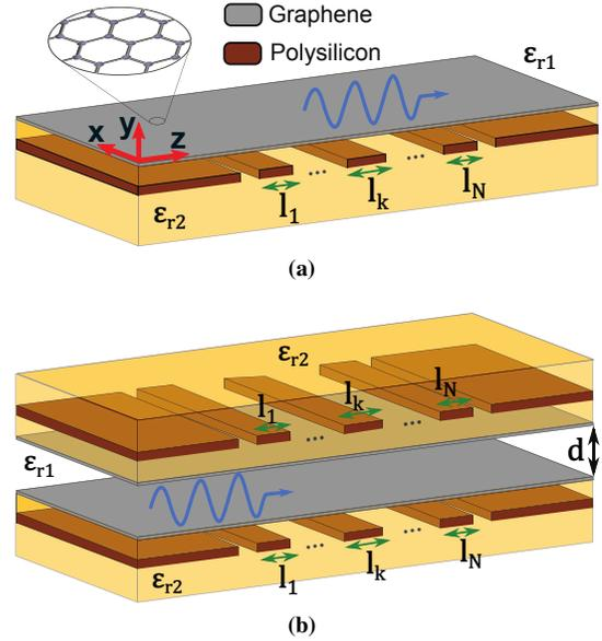
**Fig. 1:** Schematic diagram of two graphene-based waveguides. Graphene conductivity may be tuned at each waveguide section by applying a DC bias to the polysilicon gating pads. (a) Monolayer implementation. (b) PPW implementation.
