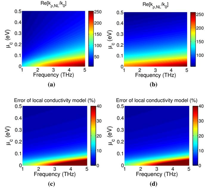
**Fig. 2:** Normalized phase constant of (a) TM mode in a monolayer graphene waveguide (see Fig. 1a) and (b) quasi-TEM mode in a graphene-based PPW (see Fig. 1b). (c)-(d) show the relative error  $100 \left| \frac{k_{\rho L} - k_{\rho NL}}{k_{\rho NL}} \right|$  in the calculation of panels (a)-(b) when using a local conductivity model. Parameters are  $d = 100$  nm,  $\tau = 1$  ps,  $\epsilon_{r1} = \epsilon_{r2} = 11.9$  and  $T = 300$  K.
