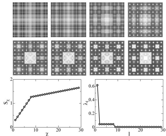
FIG. 3: (upper panels)  $M_\chi$  for  $\chi = 1, 2, \dots, 8$ , (lower left) Coarse-grained snapshot entropy as a function of  $\chi$ , (lower right) Singular value spectrum. We find that  $\lambda_1 = 0.6155$ ,  $\lambda_2 = \dots = \lambda_8 = 0.0442$ , and  $\lambda_9 = \dots = \lambda_{29} = 0.0032$ .
