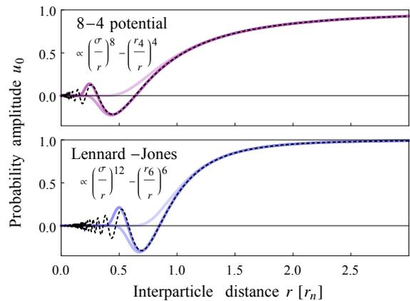
Figure 3: Pair correlation at unitarity for potentials decaying as power laws  $-1/r^n$ . Top: the 8-4 potential. Bottom: the Lennard-Jones potential. In each graph, the solid curves correspond in order of opacity to potential depths supporting respectively 1, 2, and 3  $s$ -wave bound states, which are obtained by adjusting the value of  $\sigma$ . The dashed curve represents the universal pair correlation in Eq. (4).
