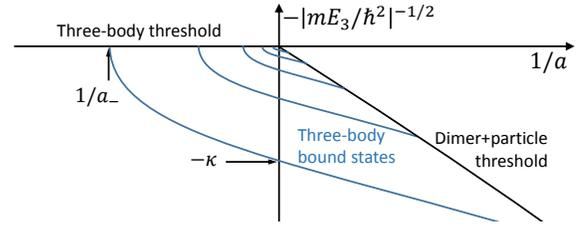
Figure 1: Schematic Efimov plot: three-body energy  $E_3$  scaled as an inverse length as a function of the inverse scattering length  $1/a$ . The arrows indicate the scattering length  $a_-$  at which an Efimov trimer state appears, and its binding wave number  $\kappa$  at unitarity ( $a \rightarrow \infty$ ), either of which serves as a measure of the three-body parameter.
