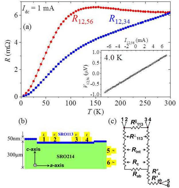
**Fig. 3.** Resistance vs temperature of a SRO113(50 nm)/SRO214 hybrid system. (a)  $R_{12,34}(T)$  (on the  $ab$ -surface; blue squares) and  $R_{12,56}(T)$  (top to side; red circles). Inset shows a linear  $I$ - $V$  curve measured in 12,56 configuration. (b) Schematic illustration of the electrodes. Top electrodes 1 to 4 are placed in a flat area away from the steps larger than the film thickness. (c) Simplified model of the resistance circuit.
