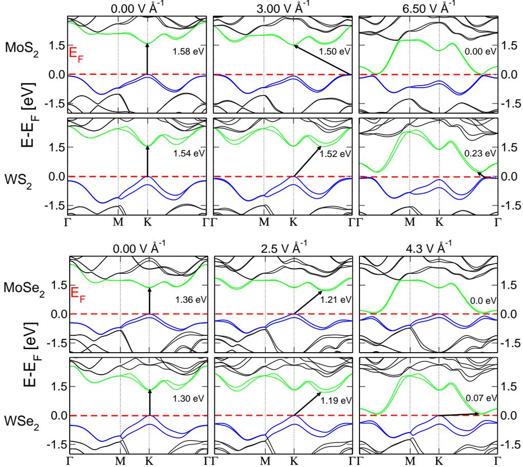
FIG. 1. Electronic band structures of  $\text{TX}_2$  systems with respect to the external electric field. The top of valence and bottom of conduction band are highlighted with blue and green, respectively. The Fermi level ( $E_F$ ) is shifted to the top of valence band. The values of fundamental band gaps are given.
