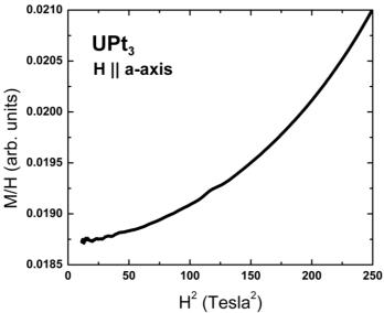
Figure 4: Shows the result of replotting the data in fig.3 confined to within a field of 16 tesla as per eqn.(10). The deviation from a straight line is clear thus indicating a significant contribution from  $\chi_5$ , the fifth order susceptibility term to the magnetization.
