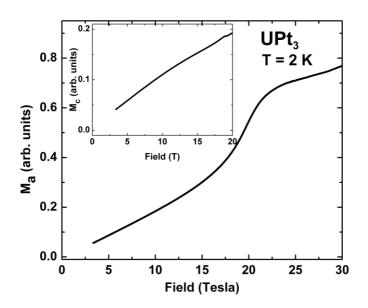
Figure 3: Shows the magnetization along the a-axis obtained after deconvoluting the torque capacitance signals in the two orthogonal directions  $\tau_1$  and  $\tau_2$  shown in fig.2. The metamagnetic transition at 20 T is clearly seen. The inset shows the magnetization along the perpendicular direction (H||c-axis).
