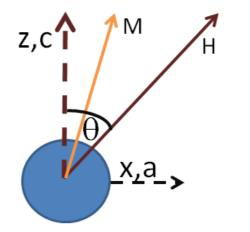
Figure 1: Schematic of an anisotropic crystalline sample placed in a magnetic field oriented at an angle  $\theta$  with respect to the c-axis of the crystal. The coordinate system is fixed to the crystal.
