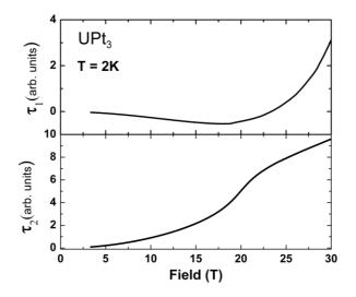
Figure 2: Shows the torque signals,  $\tau_1$  and  $\tau_2$ , obtained from a single crystal sample of UPt<sub>3</sub> when the magnetic field is applied about 1 degree away from the c-axis (top panel) and the a-axis (bottom panel) of the crystal.
