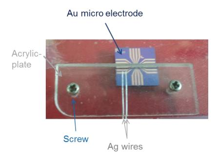
Fig. S3. A snap-shot image of experimental set-up for contact force-dependent contact resistance ( $R_C$ ) measurement. The Ag wires are connected on the same Au electrode.
