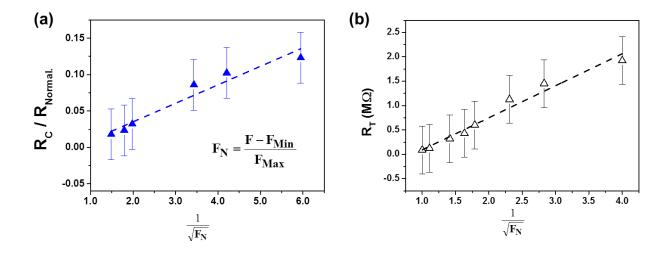
Fig. 3. Graphs of (a) normalized  $R_C$  and (b)  $R_T$  dependent on  $1/\sqrt{F_N}$ ; both show a linear correlation. The normalized applying force  $(F_N)$  is determined by the equation in (a): the  $F_{Max}$  and  $F_{Min}$  are the maximum and minimum contact force during the measurement, respectively.
