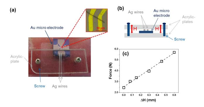
Fig. 1. (a) A snap-shot image and (b) scheme of experimental set-up for contact force dependent resistance measurement of a PPy NW device. The inset in (a) is a zoomed-in optical microscope image of PPy NW loaded area. (c) Applying force curve dependent on displacement ( $\Delta H$ ) of the distance between the acrylic plates (H).
