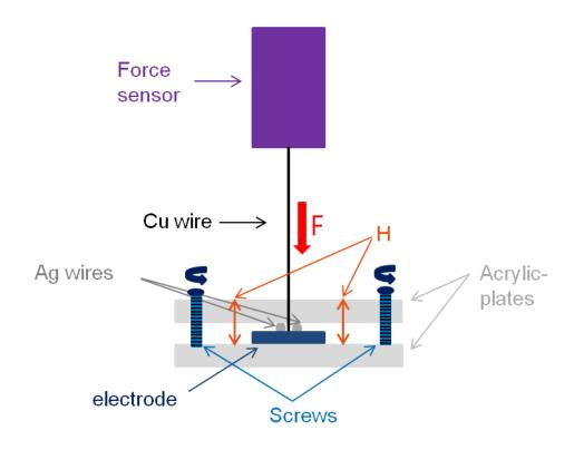
Fig. S1. Scheme of experimental set-up for contact force (F) dependent on the distance between the acrylic plates (H).
