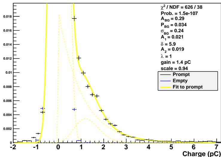
**Figure 2.** Single photoelectron charge spectrum for PMT ID PAYG at operating voltage. The data with a pulsed LED are shown in black, with statistical errors, noise data are shown in blue, and the fit model is shown in the yellow line.
