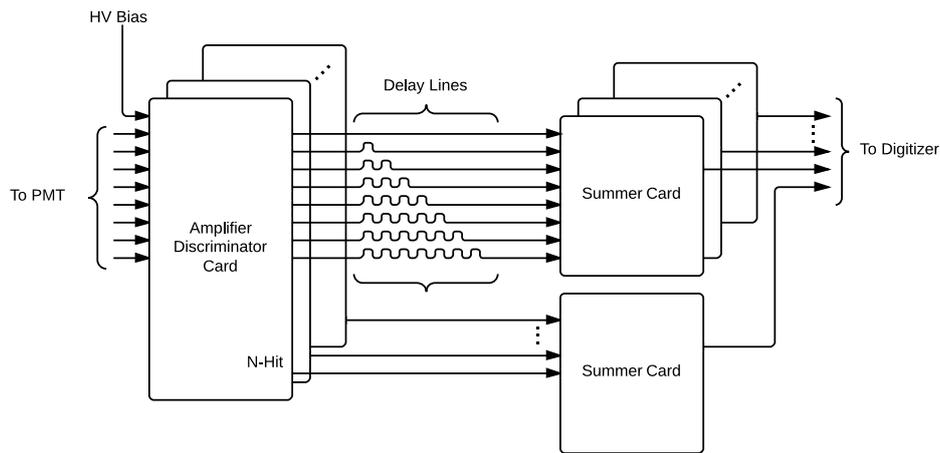
**Figure 5.** Block Diagram of MiniCLEAN Veto Electronics
