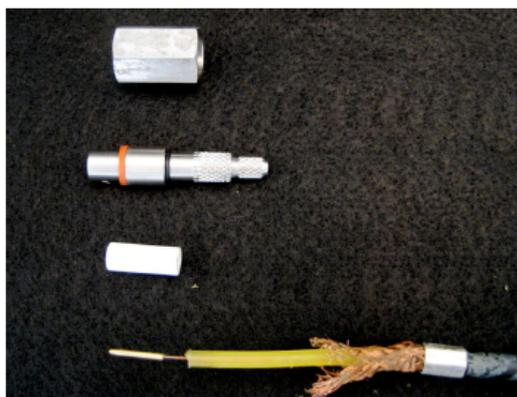
**Figure 3.** Left: TRIUMF connector assembly drawing. Items 1,2,4,6,7,10, and 11 were built or purchased to mate RG59 cable to the existing R1408 PMT jacks. Right: As-built TRIUMF connector for mating cable to the R1408 jack. From top to bottom is shown the coupling nut, the plug body into which the cable is inserted, the teflon insulator which is also inserted into the plug body, and the pin with a stripped cable.
