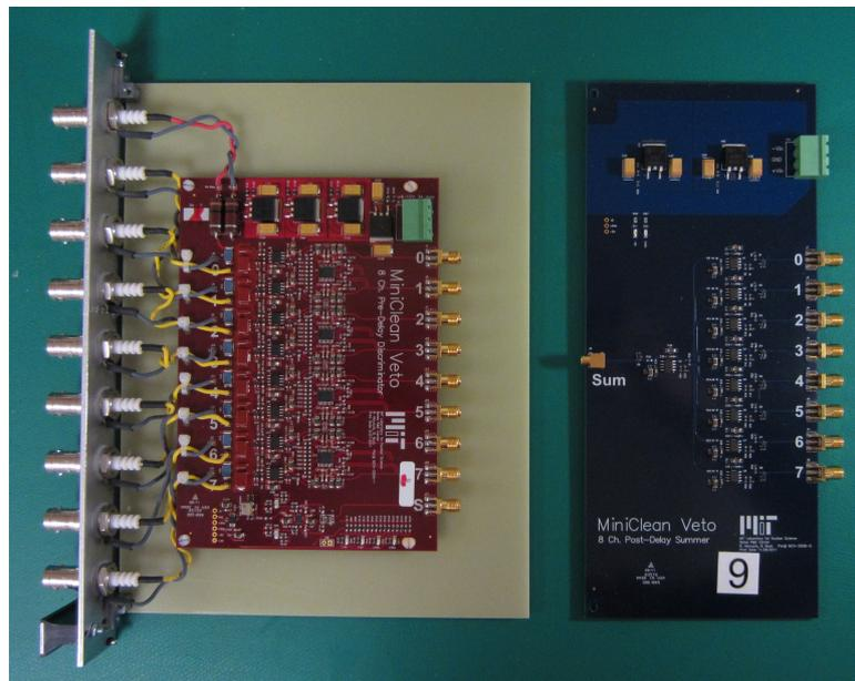
Figure 9. Amplifier discriminator board (left) and summer board (right).
