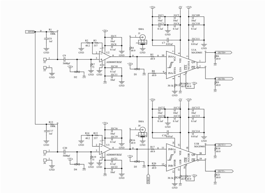
**Figure 6.** Two channels of the amplifier discriminator card. J2 and J5 make the signal connections to the PMTs. J1 and J4 make the connections to the delay lines. U2 and U3 are the amplifiers, U1 is the two channel comparator.
