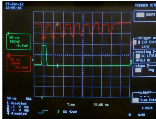
**Figure 7.** Oscilloscope capture from the output of a summer board. Eight channels pulsed with a 10 mV synchronous pulse into the amplifier discriminator board. The amplified signals are routed through the delay lines into the summer board. The top trace is the output of the summer board. The bottom trace is the N-Hit sum output from the amplifier discriminator board, used as a trigger.
