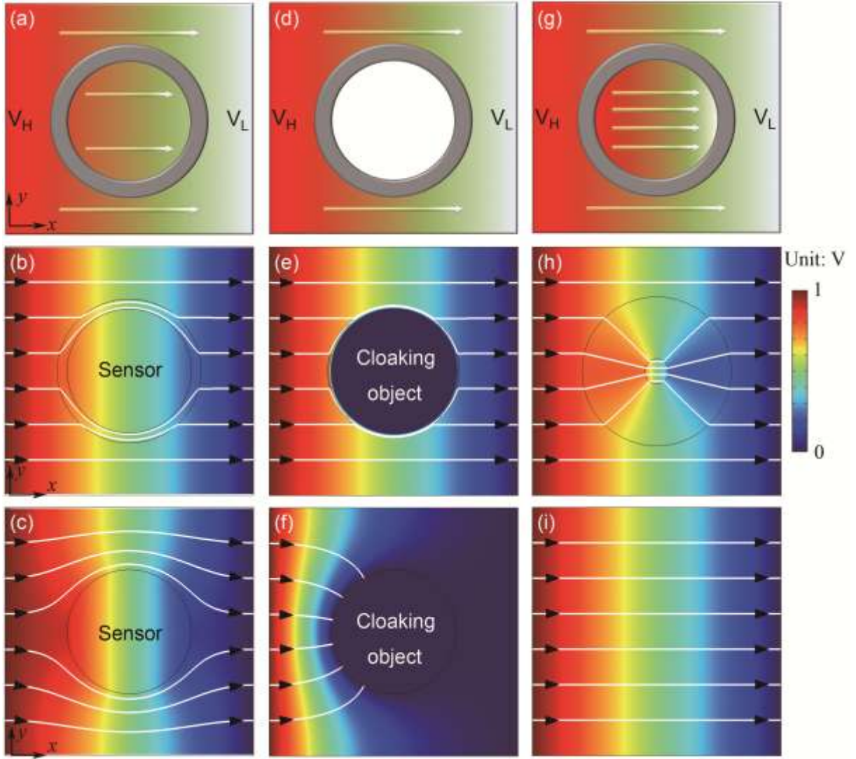
Figure 1. Demonstration of novel bilayer dc devices for manipulation of dc currents. (a) Cloaking sensor. (b) Simulation result of cloaking sensor. (c) Simulation result of a bare sensor. (d) dc bilayer cloak. (e) Simulation result of the bilayer cloak. (f) Simulation result of a bare and grounded object. (g) dc electric concentrator. (h) Simulation result of the concentrator. (i) Simulation result of a pure background without the concentrator. dc currents are represented with arrow lines in panel.
