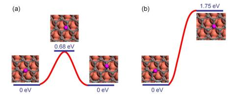
**Figure S2.** Minimum energy paths of C monomer diffusion on graphene/Cu(111) (a) between two bridge sites and (b) from bridge to top sites.
