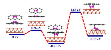
**Figure 5.** Minimum energy path of carbon dimer penetration of a graphene overlayer on Cu surface.
