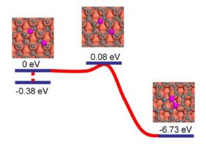
**Figure S5.** Minimum energy path of carbon monomes collision with each other to form dimer embedding in the graphene overlayer. The initial state is 0.38 eV higher than that of two carbon adatoms far away each other.
