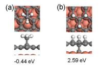
**Figure S4.** Top and side views of (a) a  $CH_3$  adsorbed on graphene/Cu(111), (b) the carbon atom in the interface. Potential energies of  $CH_3$  as defined in Figure S1 are marked in eV.
