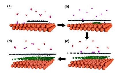
**Figure 6.** Schematic of a new bilayer graphene growth protocol. (a) A standard monolayer graphene CVD growth on Cu surface. (b) Carbon monomer intercalation via a penetration mechanism and growth of the second graphene layer. (c) Hydrogen gas is supplied to etch extra carbon species. (d) With desorption of hydrocarbons, high quality bilayer graphene is obtained.
