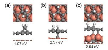
**Figure S3.** Top and side views of (a) a  $CH_2$  adsorbed on graphene/Cu(111), (b) the carbon atom in the interface, and (c) the carbon atom at a subsurface octahedron site. Potential energies of  $CH_2$  as defined in Figure S1 are marked in eV.
