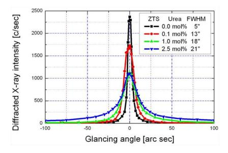
**Figure 5** Comparative representation of diffraction curves for undoped and doped (up to 2.5 mol%) specimens of ZTS crystals using (200) diffracting planes.
