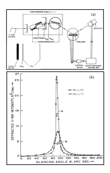
**Figure 2** (a) Schematic of the multicrystal X-ray diffractometer developed at NPL. Inset shows the MoK $\alpha$  doublet and the isolated K $\alpha_1$  beam and (b) DCs recorded in dispersive (+,-,-) and non-dispersive (+,-,+) settings.
