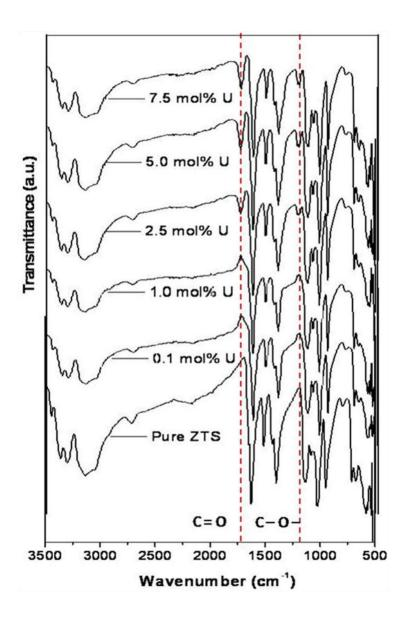
Figure 1 FTIR spectra for pure and urea (U) doped ZTS specimen.
