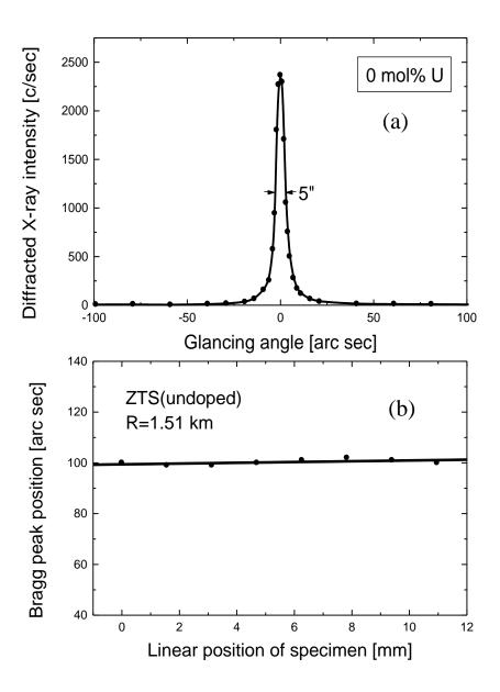
**Figure 3** (a) Diffraction curve recorded for (200) diffracting planes and (b) curvature plot of pure ZTS single crystal.
