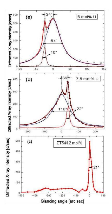
**Figure 6** Diffraction curves (a), (b) and (c) are respectively for 5.0, 7.5 and 12 mol% urea (U) doped ZTS single crystals.
