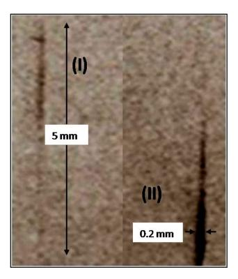
**Figure 7** Section topographs recorded at the peak positions of the DC of Figure 6(a). The topographs at I and II respectively correspond to the very low angle grain boundary (at 24 arc s away from main peak) and the main peak (at zero position).
