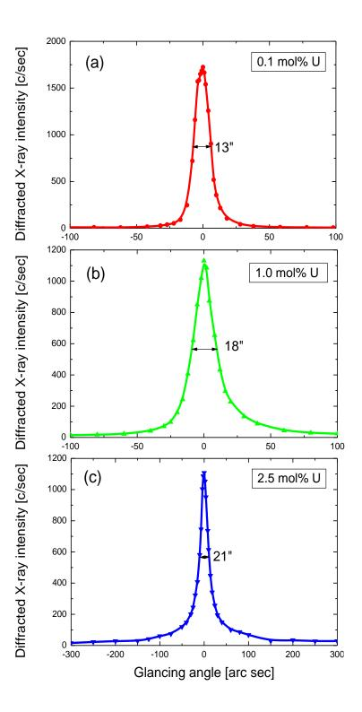
**Figure 4** Diffraction curves of doped ZTS single crystals recorded for (200) diffraction planes: (a) 0.1, (b) 1.0 and (c) 2.5 mol% urea.
