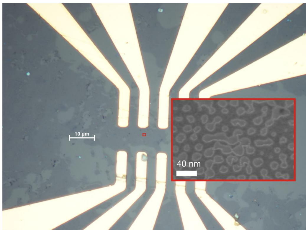
Figure S-3 Optical image of one of the device. CVD nanopatterned graphene is place on top of Gold electrodes and the polymer used for the wedged transfer is dissolved in ethyl acetate. The insert present a SEM image of the nanopatterned graphene. The electrical measurements are done using four electrodes.
