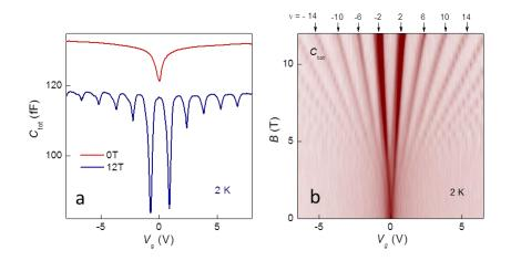
**Figure 3.** Capacitance spectroscopy of WS<sub>2</sub>/graphene/hBN/Au. (a)  $C_{tot}$  as a function of  $V_g$  in zero and quantizing *B*. For clarity, the 12T curve is offset by 15 fF. (b) Landau fan diagram  $C_{tot}(V_g, B)$ . Scale: wine to white 0.105 to 0.120 pF.
