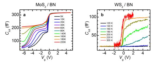
**Figure S5.** Capacitance spectroscopy of MoS<sub>2</sub> and WS<sub>2</sub>. (a) Capacitance  $C_{tot}$  as a function of bias  $V_g$  for a typical MoS<sub>2</sub>-based capacitor device (without graphene on top). (b) Capacitance measurements for a similar WS<sub>2</sub>-based device.
