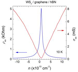
**Figure S2.** Resistivity and conductivity in zero *B* for the graphene-on-WS<sub>2</sub> Hall bar device.
