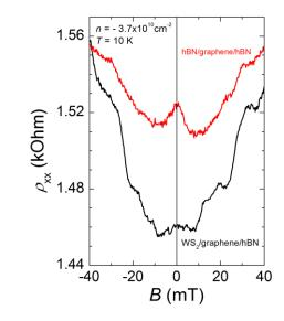
Figure S3. Comparison of the small-field magnetoresistance obtained from the graphene-on-hBN (red curve) and graphene-on- $WS_2$  (black curve) devices measured at the same carrier concentration.
