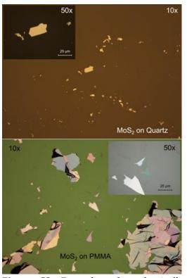
**Figure S2.** Examples of mechanically exfoliated  $MoS_2$  flakes on quartz (top) and PMMA (bottom) substrates. The yield of exfoliation is very similar to that of graphene.  $WS_2$  demonstrates very similar behavior.
