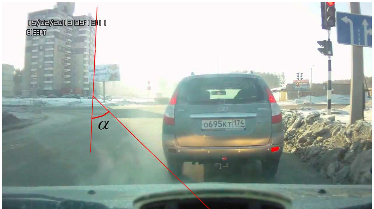
Figure 1. The shadow from the arris is on the horizontal road surface. The angle \alpha is sensitive to the azimuth of the bolide and takes on a zero value at the moment of conjunction of azimuths of the bolide and the arris.
