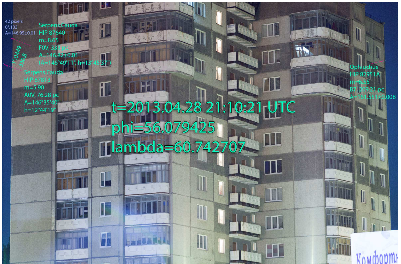
Figure 5. The determination of the azimuth of the arrises by stars HIP 87640 and HIP 82951A. The azimuth of the left arris is equal to the 146.95^{\circ} \pm 0.01^{\circ} , the azimuth of the right arris is equal to the 161.551^{\circ} \pm 0.008^{\circ} . The distances to the arrises are equal to 143 m and 161 m accordingly.
