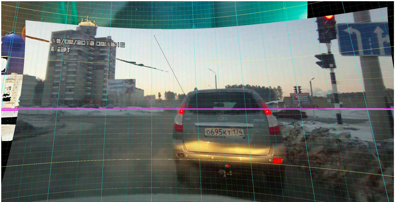
Figure 6. The example of superimposing of the alt-azimuth grid. Firstly, the parameters of the calibration frame with the sky of stars are determined, and then the frame from the video record is set with the calibration frame in the picture outlines, with that the alt-azimuth grid is superimposed.
