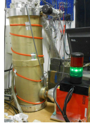
Fig. 4 (Color online) The micro-focus X-ray source in front of the CEB cryostat.
