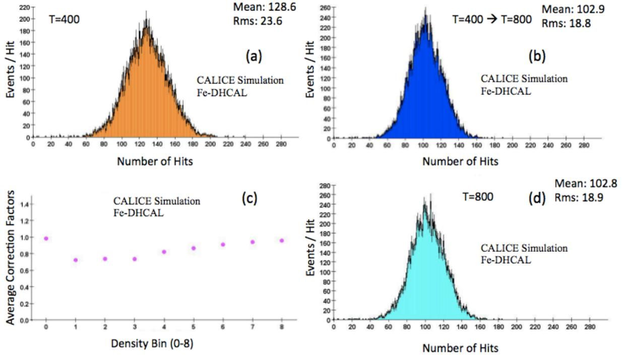
**Figure 1.** Demonstration of the density-weighted calibration procedure using 10 GeV pion MC sample digitized with two different thresholds  $T_1=400$  and  $T_2=800$ . (a) Response at  $T_1=400$ , (b) corrected response at  $T_1=400$  to obtain the response at  $T_2=800$ , (c) average correction factors as a function of the density bins (0-8) and (d) the original response at  $T_2=800$ .
