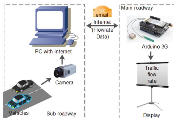
Fig. 1: Traffic monitoring system architecture
