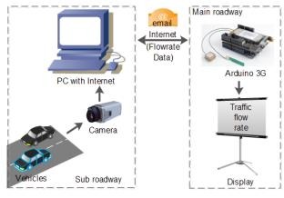
Fig. 1: Traffic monitoring system architecture
