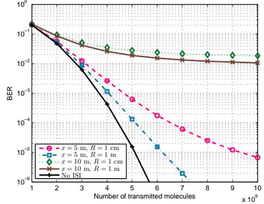
Fig. 4. BER plot for molecular communications, with Gaussian noise and with or without ISI at different transmission distances  $x$  and capture zone sizes  $R$ . The constant parameters is  $T_s = 3$  s,  $\tau = 0.5$  s, and  $v = 5$  cm/s.
