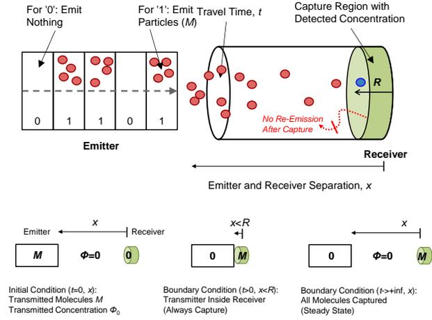
Fig. 1. Illustration of molecular communication link using On-Off-Keying (OOK) modulation scheme with a receiver that has a capture radius of  $R$ . Three conditions are presented: i) initial pulse transmission ( $t = 0$ ), ii) always full capture ( $x < R$ ), and iii) infinite capture ( $t \rightarrow +\infty$ ).
