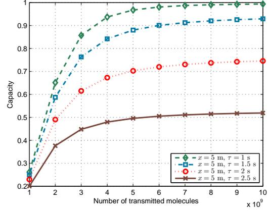
Fig. 7. Throughput plot for molecular communications with Gaussian and ISI noise with different sensor cleanse durations  $\tau$ . The constant parameters are:  $T_s = 3$  s,  $v = 5$  cm/s, and  $R = 1$  cm.
