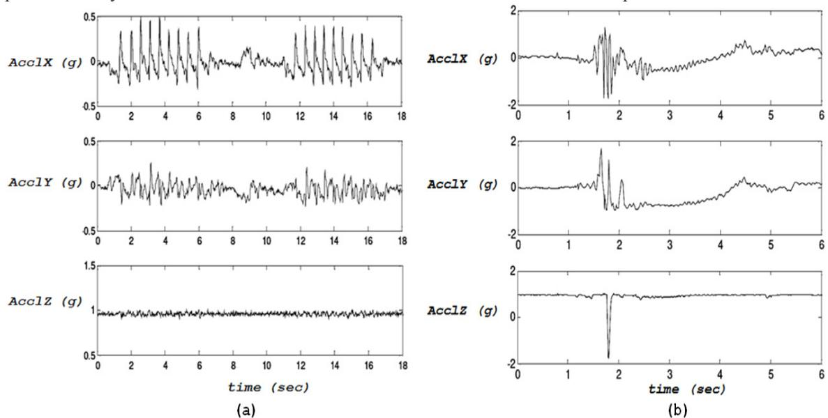
Fig 3. Accelerometer measurements showing (a) walking (ID – 2) and (b) falling (ID – 4)
