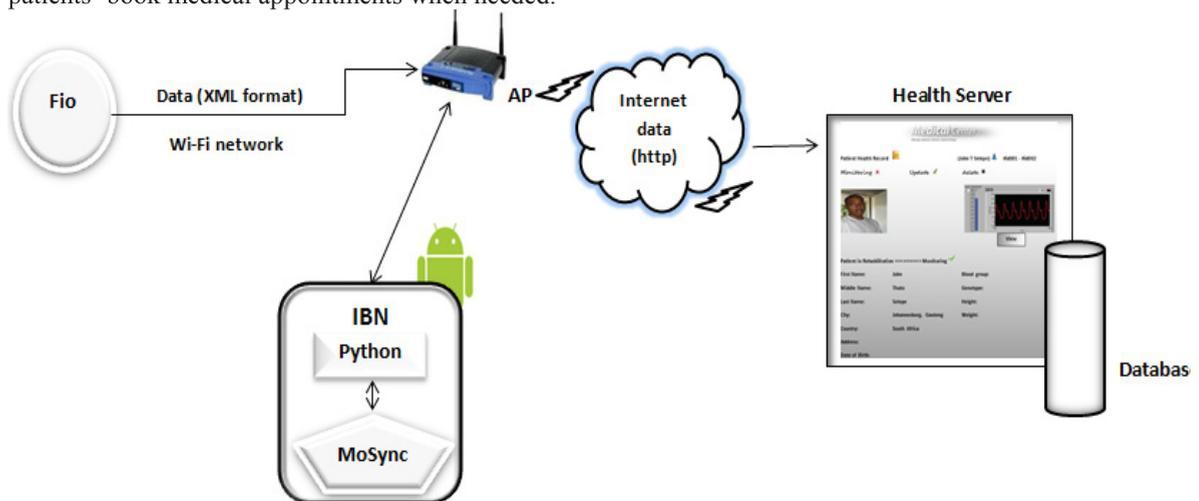
Fig. 2. Prototype WUHS data transmission process
